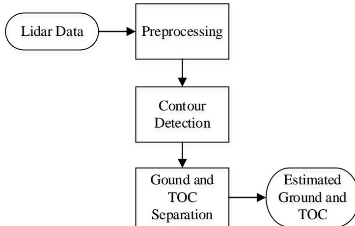
Figure 1: Overview of system. The goal is to detect curves that correspond to the ground and to the top of the canopy (TOC).
