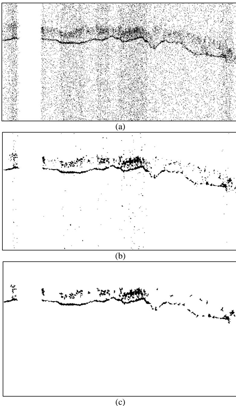
Figure 2: Example of noise reduction steps. (a) Original lidar data. Each dark point represents a single lidar measurement. (b) Result of median filter. (c) Result of size filter. For this example, the points that remain are near the ground and vegetation.
